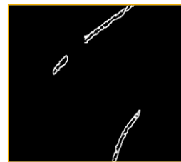
Figure 17. Removal of noise through small blob finding.
