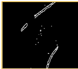
Figure 18. Edge detection with barrel obstacle removed, some noise remains.
